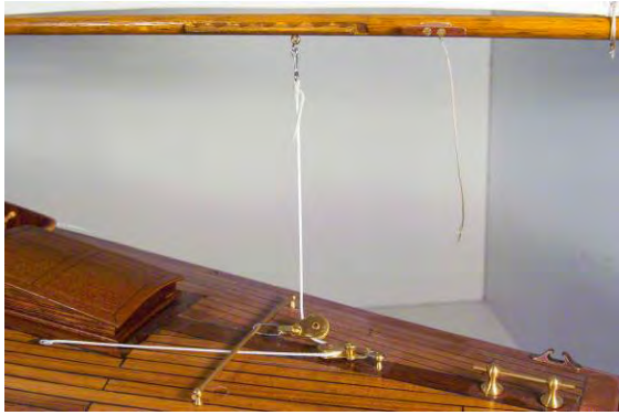
Installing the headsail winch
